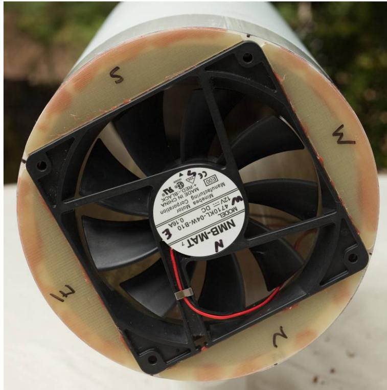
Figure 6. Fan Mounting
