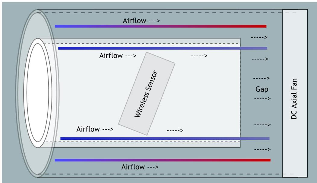
Figure 1. Coaxial Shield Concept
