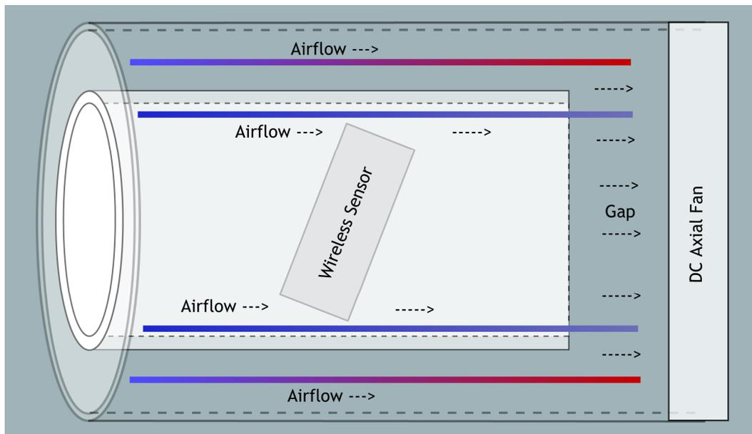
Figure 1. Coaxial Shield Concept
