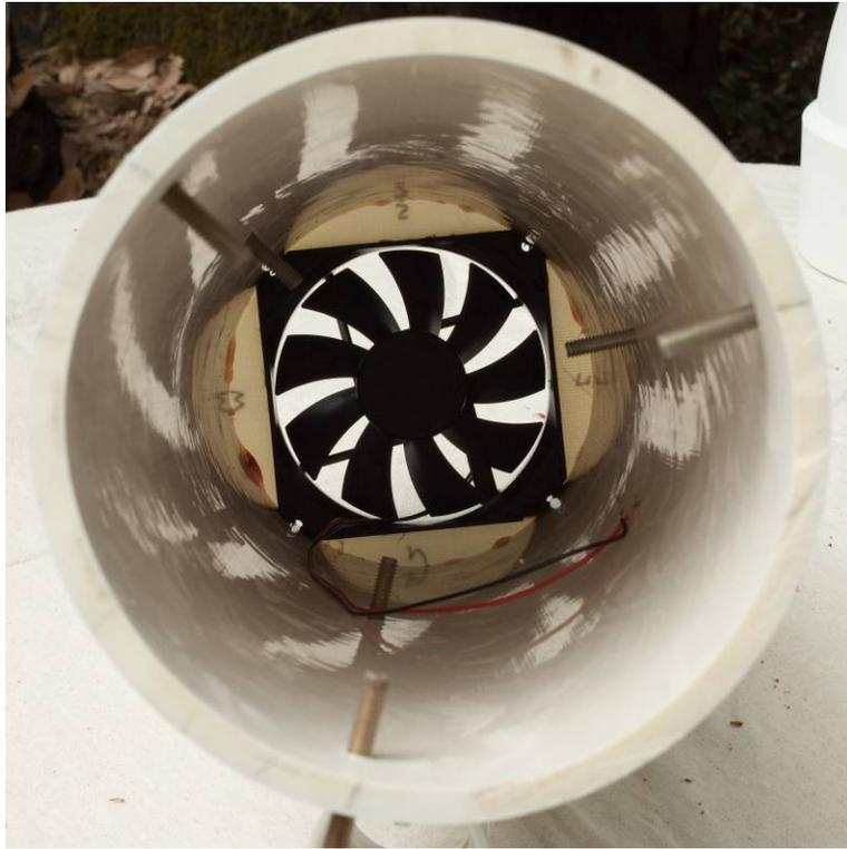
Figure 7. Mounting Screws for Inner Pipe
